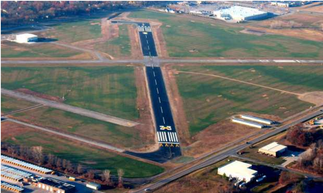
Figure 2-1 Markings for a Temporarily Closed Runway
