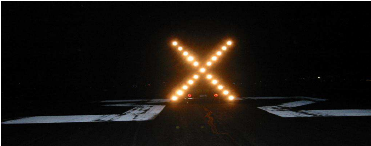
Figure 2-4 Lighted X at Night
