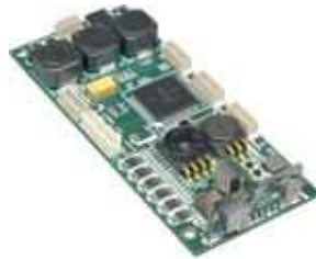
Figure 12: Phoenix O-Navi Integrated IMU/GPS (O-Navi, 2006)
