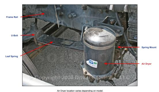
Located either behind the front bumper or behind the fuel tank.
