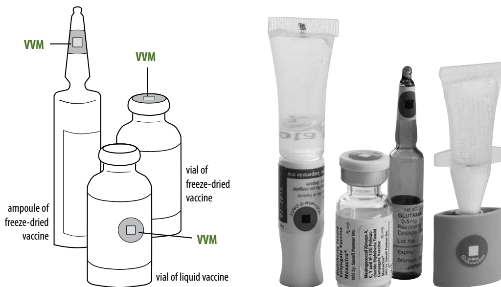
Figure 2.11 Location of VVMs on ampoules and vials
