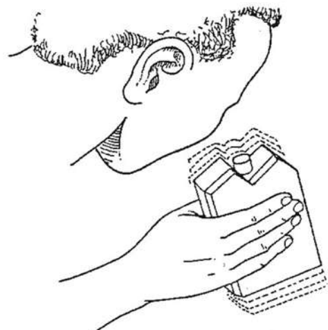
Figure 2.23 Checking that an ice pack is properly conditioned
