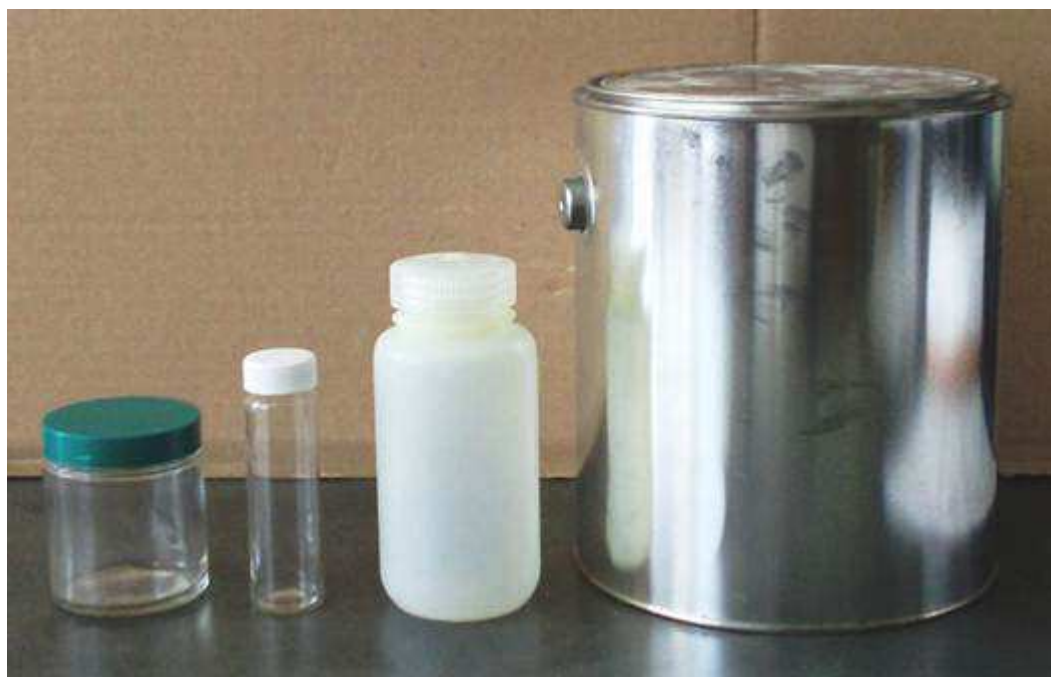
Figure 8: Sample containers for collection of liquid samples at clandestine laboratory sites. Approved containers include glass jars with Teflon-lined screw caps, plastic jars with screw caps, and metal paint cans.
